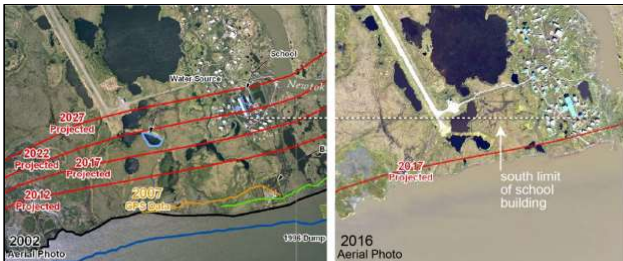
Figure 5. Comparison of projected erosion rates, with the shoreline position as of September 2016 (left, ASCG 2004; right, 2016 aerial photo courtesy of USGS)
