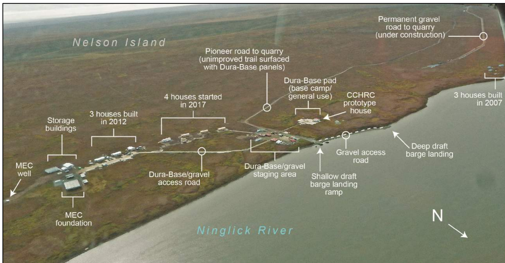
Figure 14. A September 1 st , 2017 aerial photograph of the Mertarvik project site viewed from the northeast, with existing infrastructure identified in annotations.
