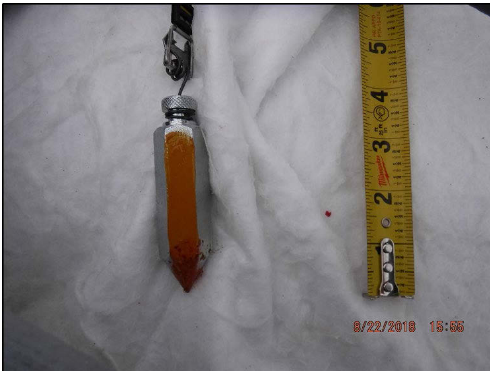
Photograph 4: Plumb bob with water indicating paste after being dropped into Tank S1.
