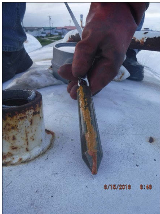
Photograph 13: Water finding past showing 1 inch of water in Tank #11.
